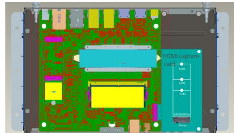
Modular Design: Motherboard + HDMI Capture Card
